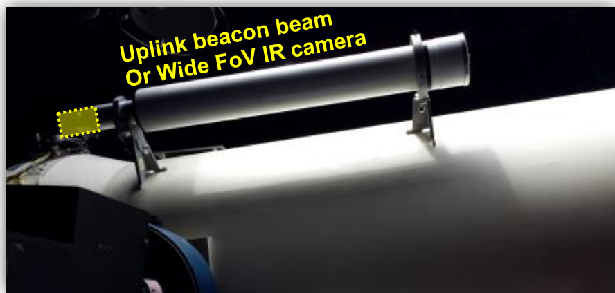
Wide FoV Camera (1700 arcsec) installed on 200 mm telescope mounted on MeO
