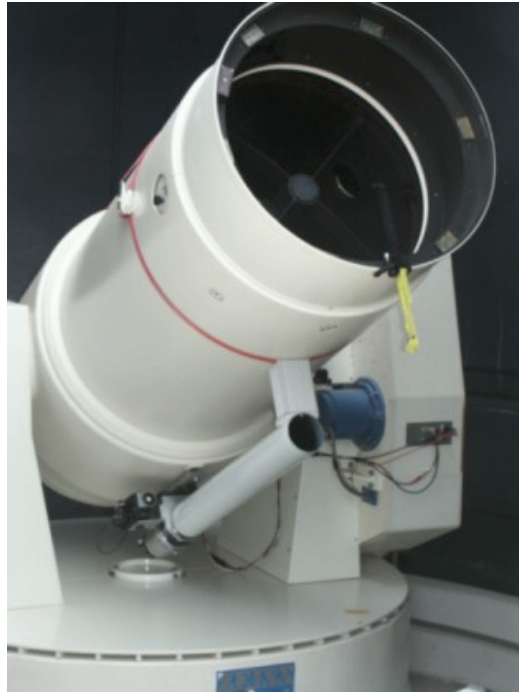
Figure 4.1-15. Second aperture at the WLRS to measure very low orbiting satellites.
