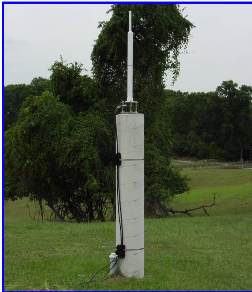
Figure 5. DORIS GREB antenna on the pillar monument
