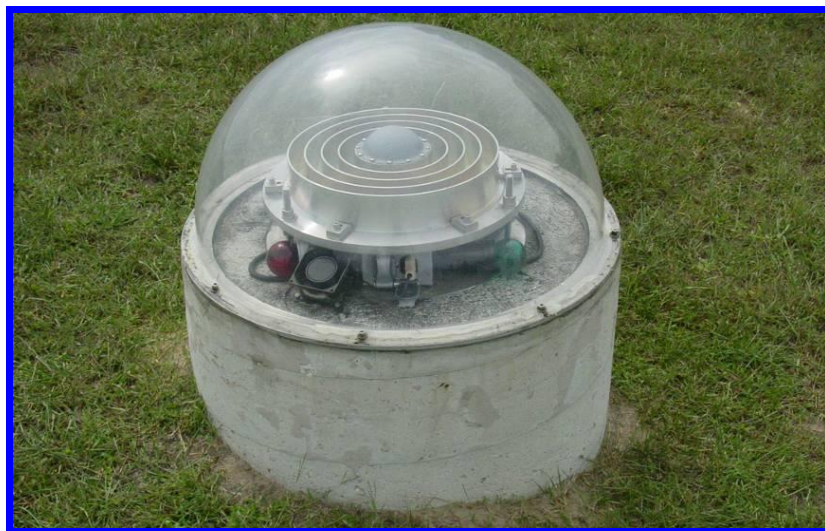
Figure 4. GPS GODE antenna on pier monument
