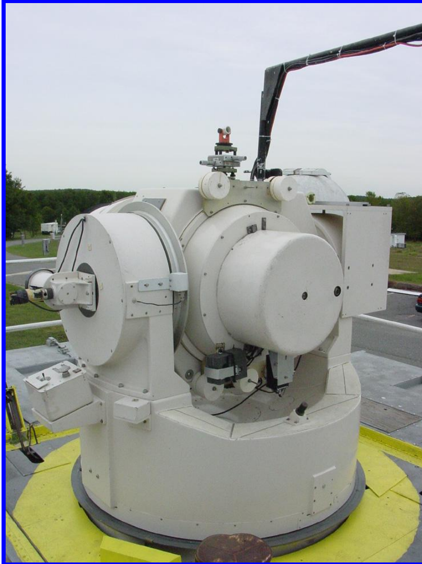
Figure 10. Translation Stage on MOB LAS 7 Telescope
