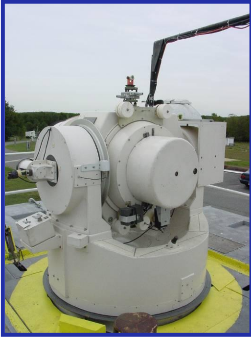
Translation Stage with Survey Prism on SLR Telescope
