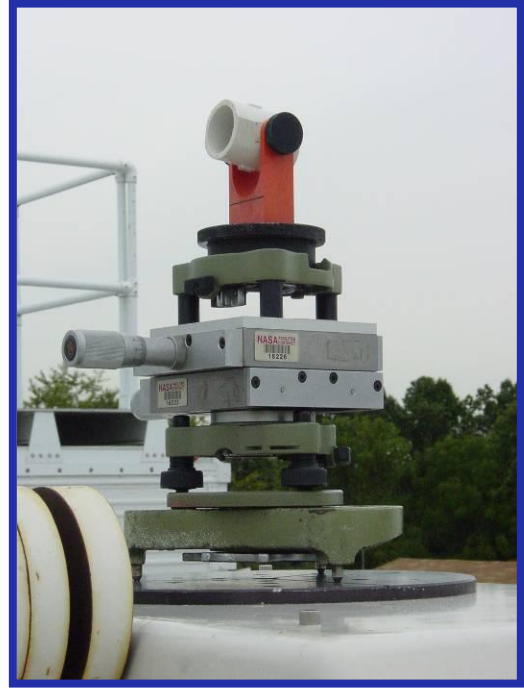
Close View Translation Stage and Prism on Trivet Plate
