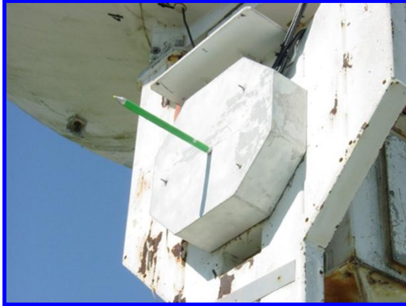
Figure 9. Close View of VLBI Antenna Elevation Axis Target
