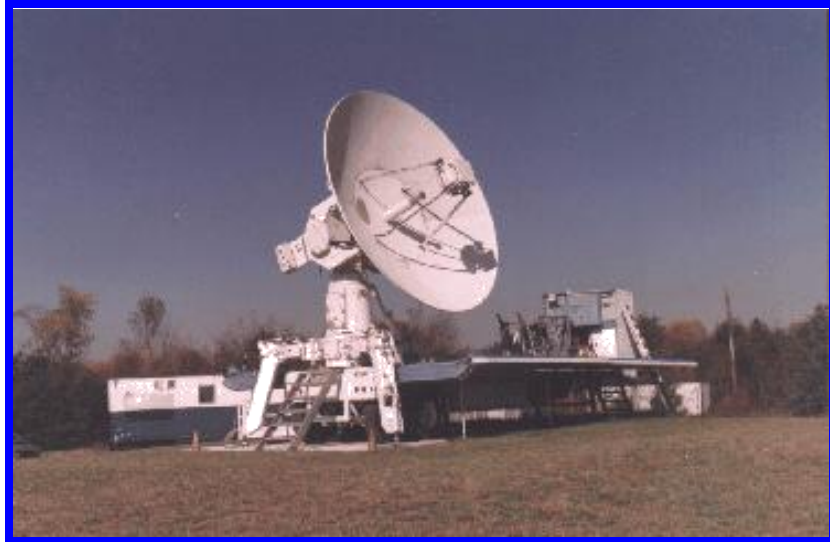
Figure 1. Global View of VLBI 5-meter Antenna in Transportable Configuration
