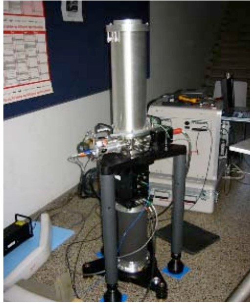
Absolute gravimeter (FG-5), capable of 10^{-9} accuracy within a few hours usually 1 day measurement. Local environmental effects are the main limitation in accuracy of such measurements
