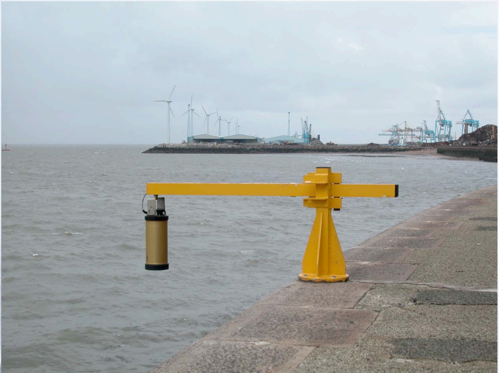
Radar gauge test installation at Liverpool
