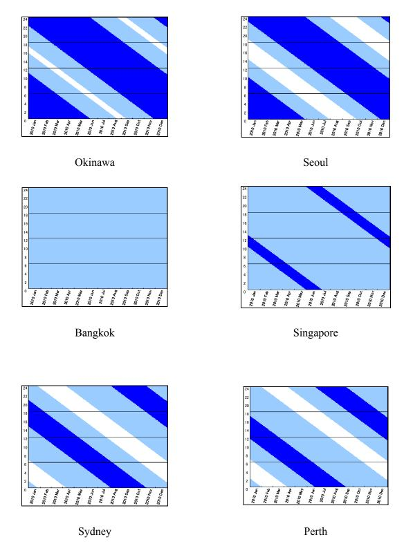
Figure 1.5.3: Initial Single-satellite QZSS visibility time for eight reference locations (dark shaded areas represent elevation angles of 60° or more; light blue areas represent elevation angles of 10° to 60°; vertical scale is hours)
