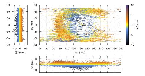
**Figure 5.** Color-coded de-meaned SLR range residuals determined using the ROCK SRP model [*Fliegel et al.*, 1992]. The residuals are projected into a coordinate system where  $\beta$  is the elevation above Sun above the satellite's orbital plane and *u* is the argument of latitude of the satellite relative to that of the Sun. After *Flohrer* [2008].
