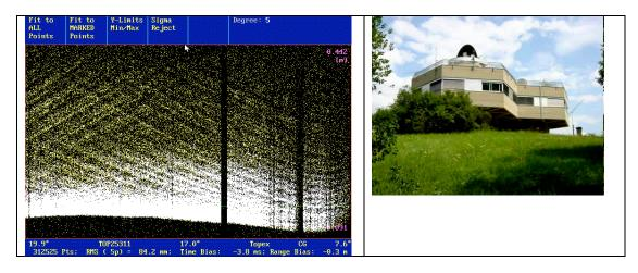
Figure 1 2 KHz returns from Graz Station with a 35 ps pulse width on the TOPEX Satellite (provided by Georg Kirchner)
