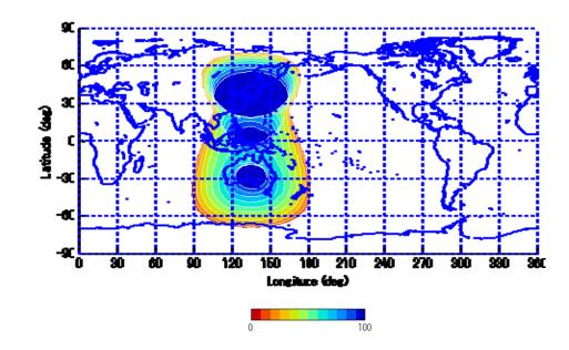
Figure 1.5.2-2: Percentage of time during which at least one QZS in the 3-satellite QZSS constellation can be seen at an elevation angle of  $60^{\circ}$  or more
