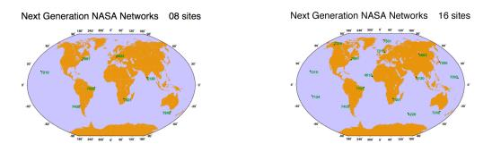
Figure 4. The two networks of SLR tracking stations examined in this study.
