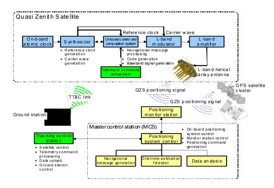
Fig.1.3-1 Configuration of the QZSS system
