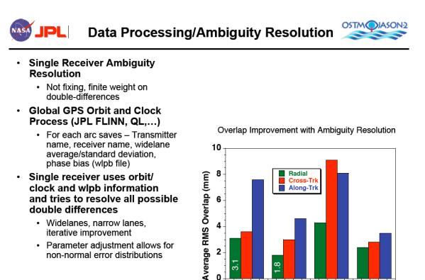
**Figure 2.** Orbit overlap RMS for Jason-2, based on improved ambiguity resolution [Bertiger et al., 2009].
