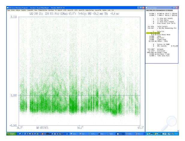
Figure 1b 2 KHz returns from Graz Station with a 35 ps pulse width on the Lageos 2 Satellite (provided by Georg Kirchner)
