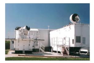
**Figure 6** The NASA MOBLAS-5 SLR system in Greenbelt, Maryland; the aircraft RADAR is at top-right
