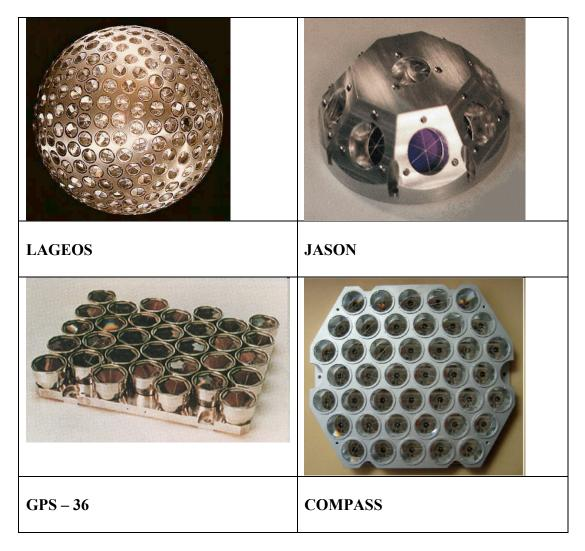
Figure 3 Examples of Retroreflector Arrays (From the ILRS website)
