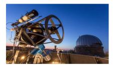
Uhlandshöhe Research Observatory, Stuttgart's first SLR station, using a fibre transmitter and a 100 kHz ranging laser.
