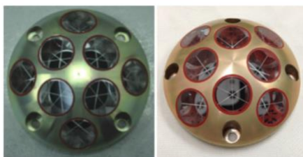
Figure 7-37. Left: microreflector payload for ESA ExoMars 2016. Right: microreflector payload for NASA InSight 2018.
