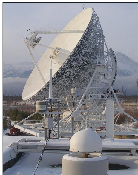
Figure 8-18. GNSS antenna, DORIS antenna and RT-32 radiotelescope.
