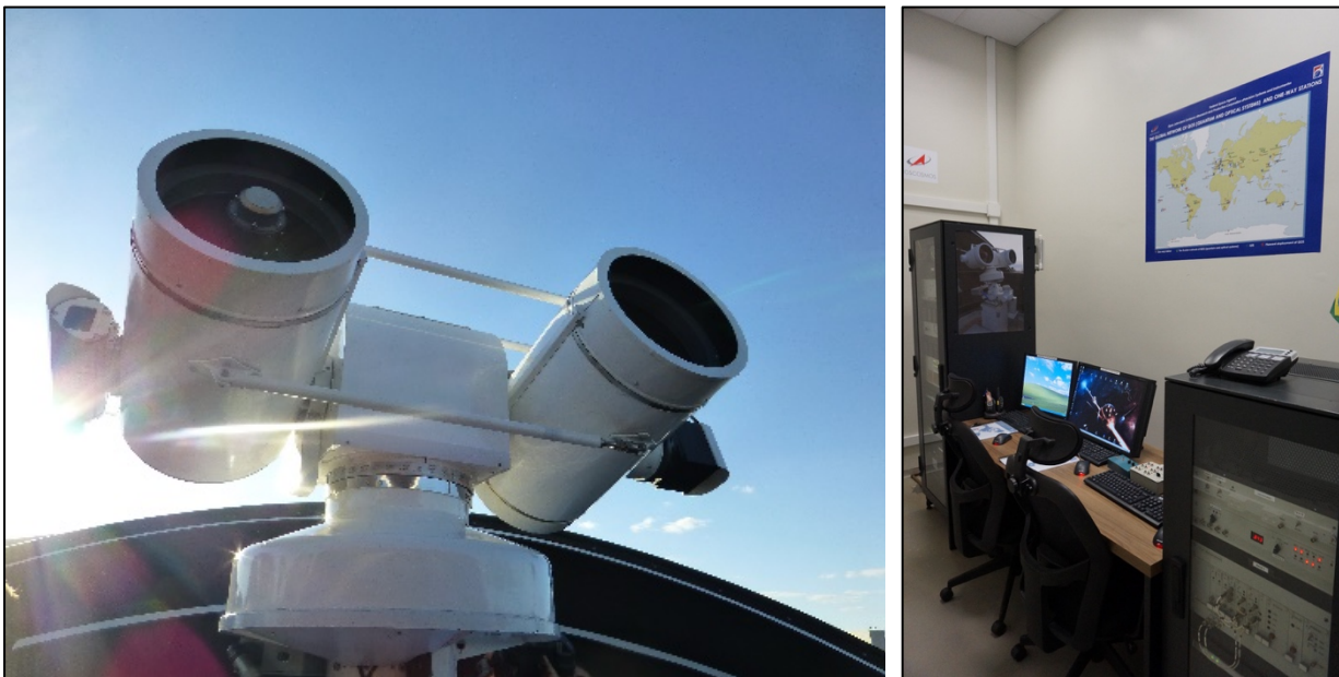
Figure 8-23. SLR telescope and operations room at Brasilia, Brazil.
