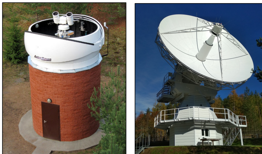
Figure 8-83. The SLR system building (left) and VGOS antenna of RT-13 radiotelescope (right).
