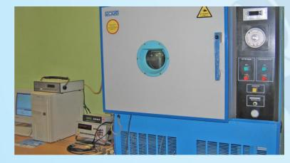
Stationary calibration complex for air humidity sensors
