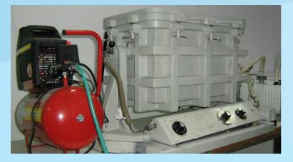
Stationary calibration facility for atmospheric pressure measuring instruments
