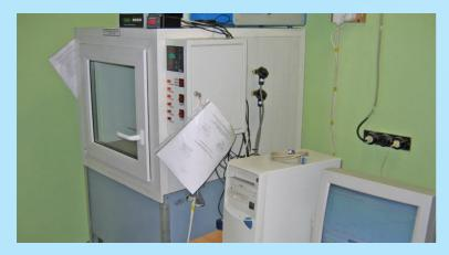
Stationary calibration complex for air temerature sensors
