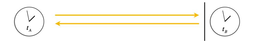
We send a light pulse at  $t_A$  from clock A to clock B, which is detected and reflected at clock B. It returns back to clock A at  $t'_A$ . The time of arrival at clock B in the timescale of clock A can be computed as:
