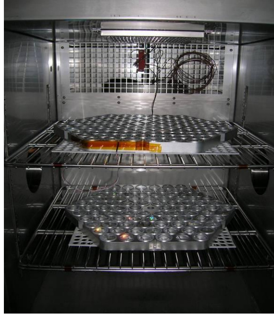
Figure 4. Environmental testing of LRA
