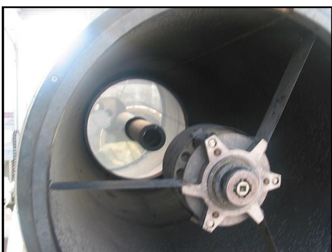
Figure 1: The 0.3 m mirror and spider mounted on the 1 m telescope.
