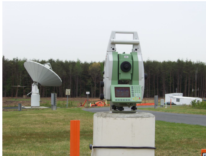
Figure 4: The Robotic Total Station at GGAO that is part of the site's Vector Tie System.
