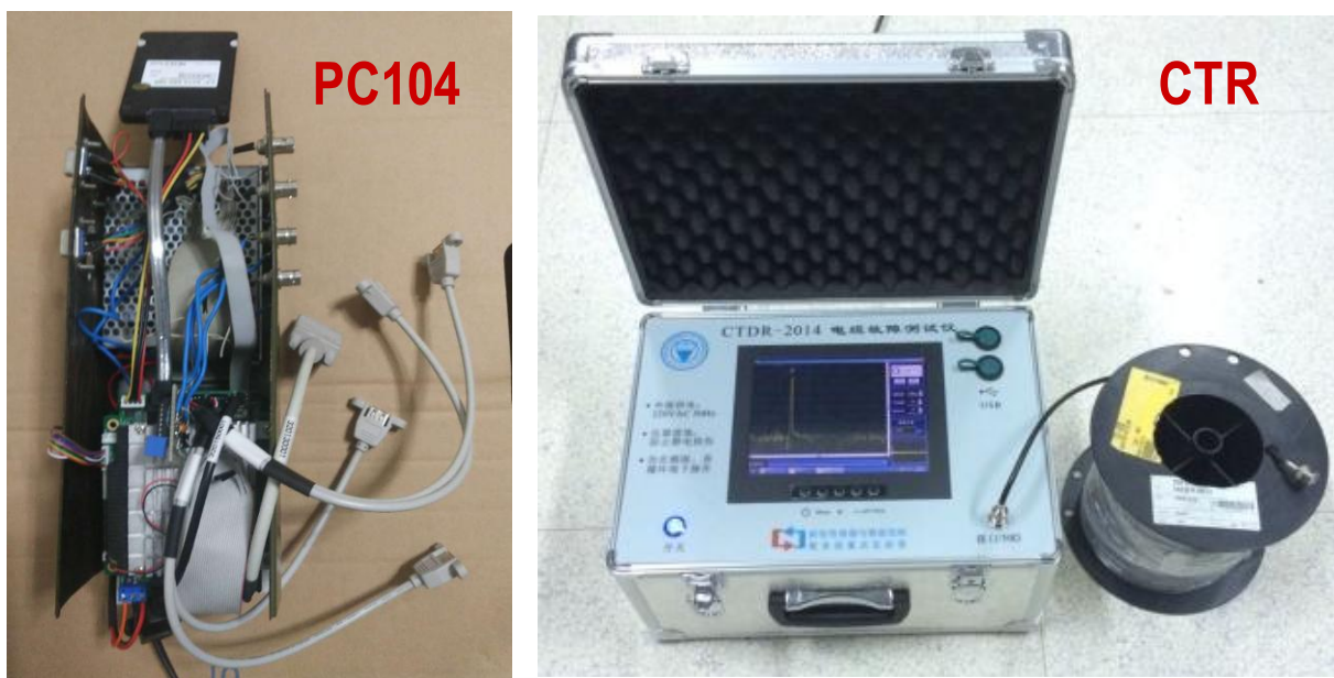
Fig.6 PC104 for servo control and equipment for checking the connectivity of cable line
