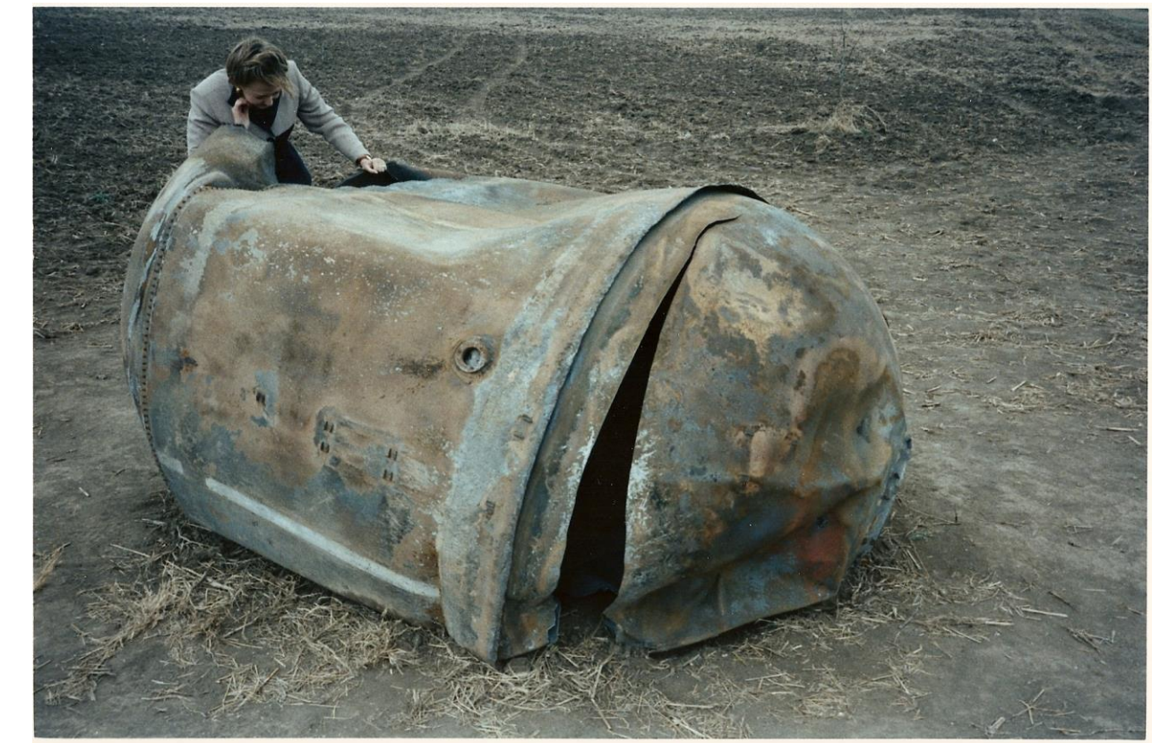
The main propellant tank of the second stage of a Delta 2 launch vehicle landed near Georgetown
