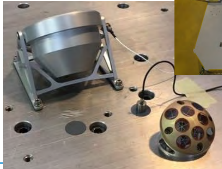
Porcell et al., Lunokhod vs. MoonLIGHT retroreflectors
